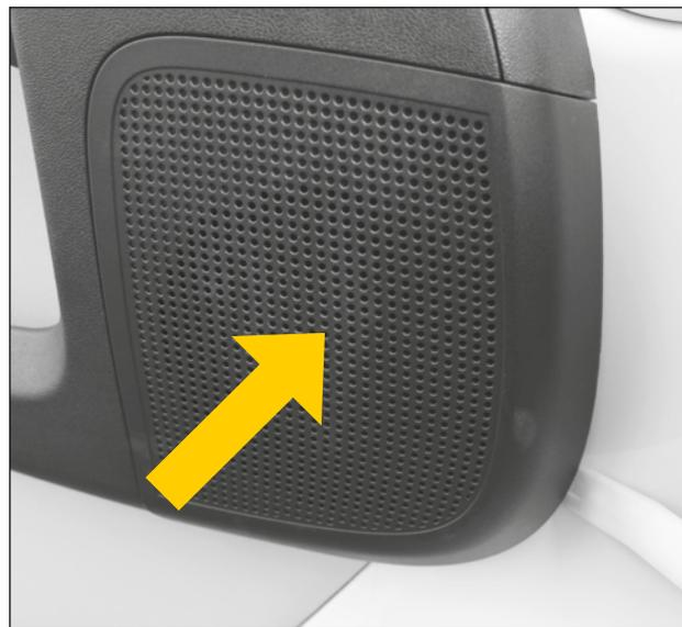
To install the tweeter, remove the cover of the a-pillar by pulling. If your vehicle is equipped with a front window curtain, you have to loosen the horizontally sliding rail before.
