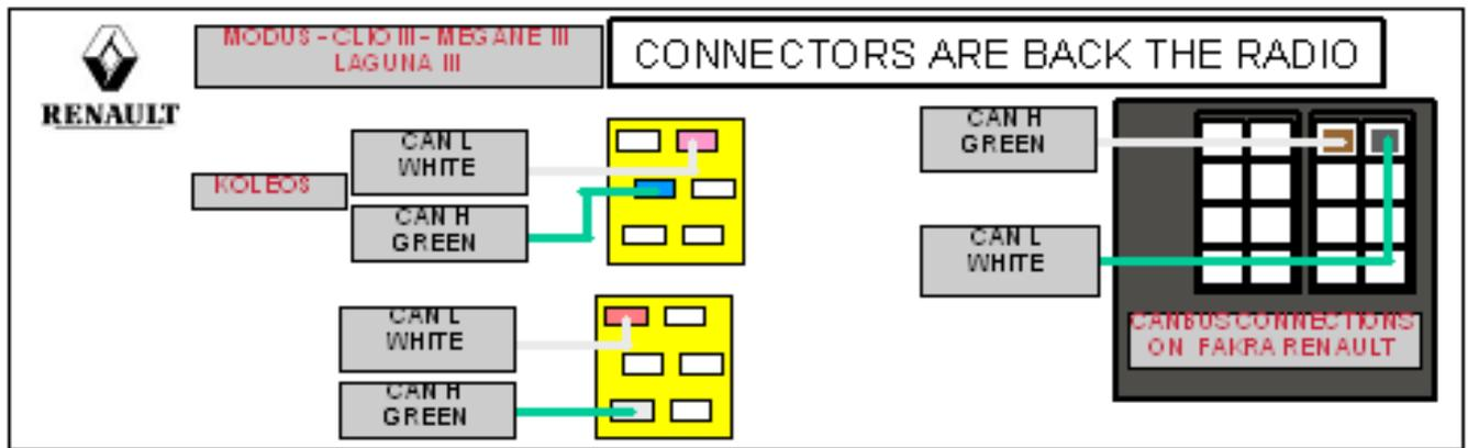
**!!!ATTENTION IN DODGE NITRO THE CAN BUS WIRES COULD BE SWAPPED IN THE VEHICLE!!!**
