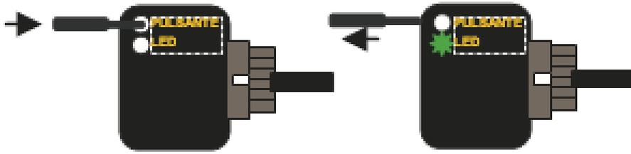
4. The LED of the interface start to blink GREEN, by making 1 flash follow by a pause. Now following the sheet to choose the function you need. Each time the interface button is pressed the flashes of the LED increase.
