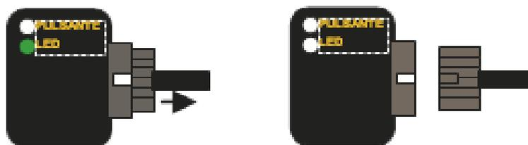
2. Press and keep pressed the button of the interface, than reconnect the cable kit.
