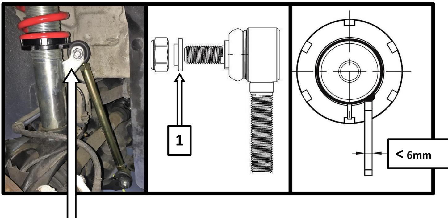
**🇬🇧 IMPORTANT NOTE :** 1 reduction ring is used on a stabiliser or stabiliser bracket, if the stabiliser or stabiliser bracket has a thickness up to 6 mm.
